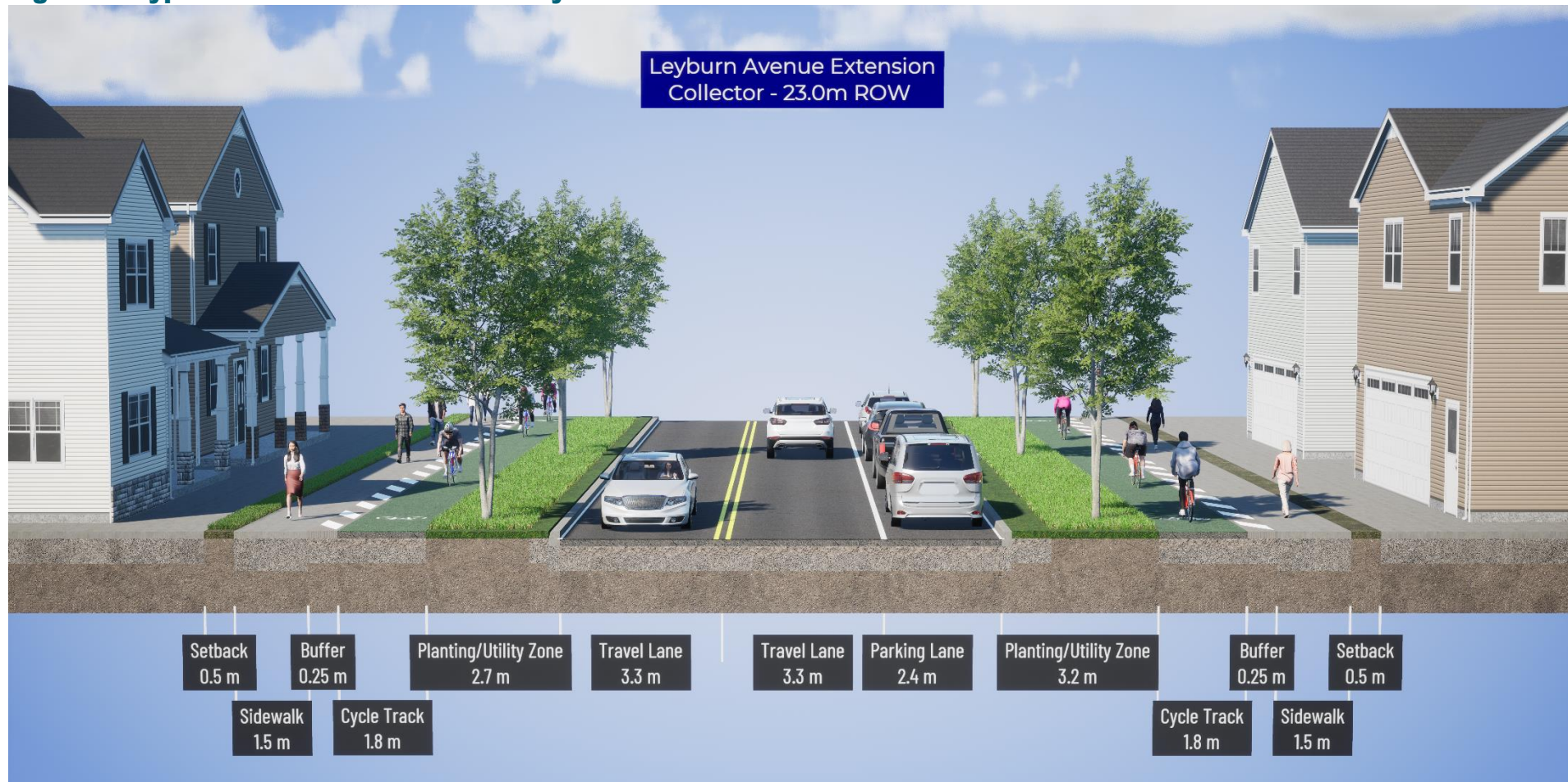
Figure 1. Typical Road Cross-section – Leyburn Avenue Extension
